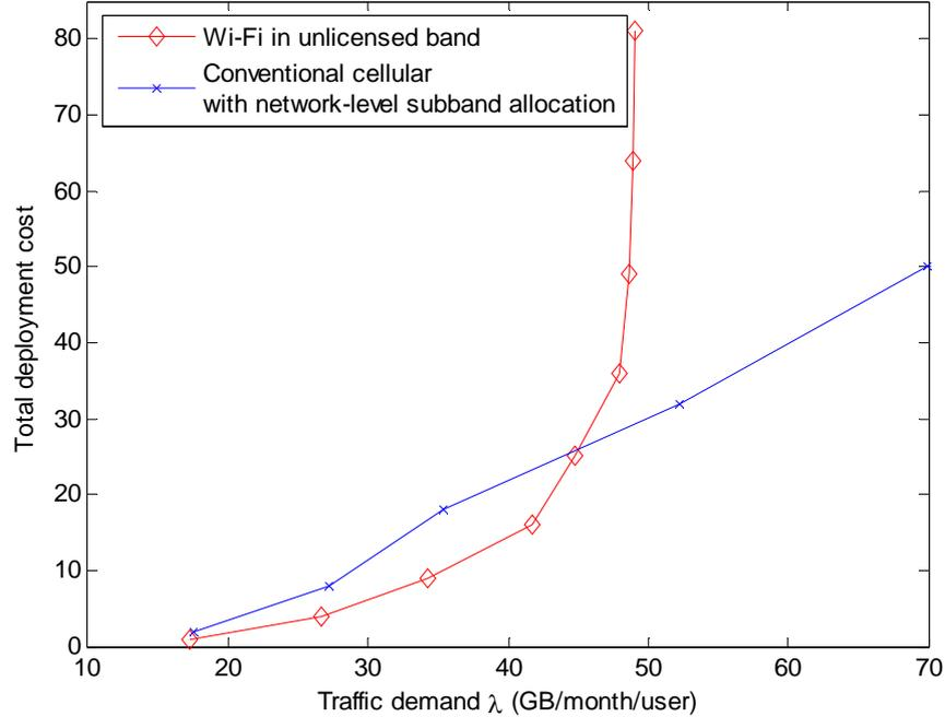
Figure 5. Total deployment cost comparison between Wi-Fi in unlicensed band and a conventional cellular system. The cellular system is assigned the half of spectrum by 3<sup>rd</sup> party spectrum broker to avoid inter-building interference while Wi-Fi system fully access whole spectrum based on CSMA/CA.
